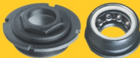
SE-502-A B.B. CUP BSA TYPE THREAD : 34.80x24 TPI FINISH : ZP / BLACK to order
