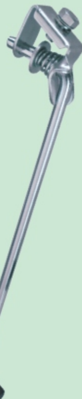
SE-3300-C-01A CENTRE STAND WHEEL SIZE : 16", 20" with Hex Bolt / Allen Bolt FINISH : Black / BCP to Order
